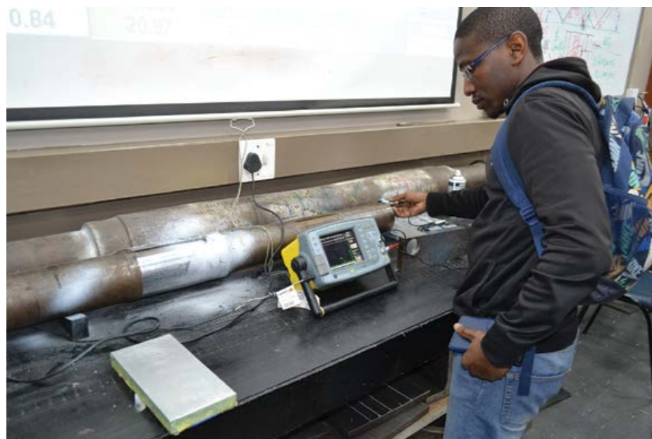
At an open day at SAIW, NDT bursary candidates look for a weld flaw in a pipe weld using ultrasonic testing (UT).
