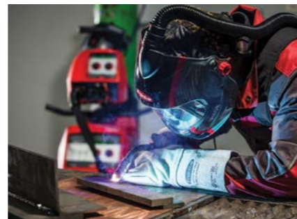
Pulse welding helps the welder to produce neat seam rippling or to minimise distortion, such as during tacking.
