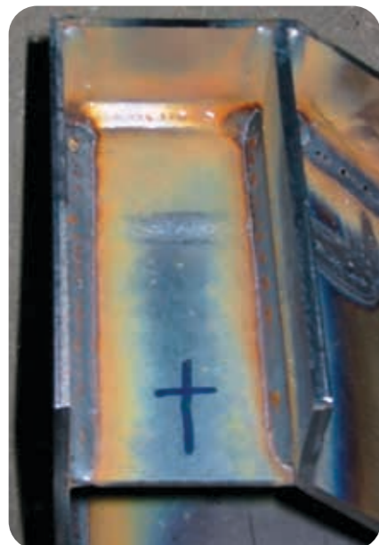
In weld trials conducted at Air Products to compare a two part argon/CO 2 mix and Air Products’ MagMix3 three-part mix with CO 2 in the 5% range, the welding time for a 30 cm weld was reduced from 58 to 48 seconds when using MagMix3, while producing a cleaner weld with less spatter that required less post-weld grinding.
