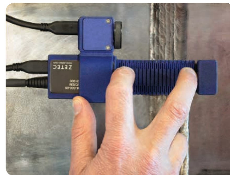
The Surf-X Array Probe can handle a range of inspection applications, from inspecting corrosion or cracking in pipes, pressure vessels, or tanks, to assessing and sizing cracks in raised welds and friction stir welds.
