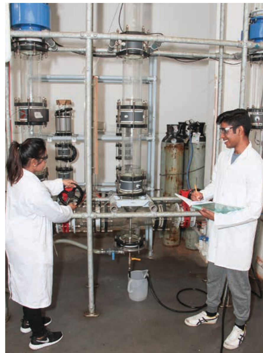
A dual airlift reactor being used at DUT to investigate the effects of change in flow area. Airlift reactors have no moving parts and provide a sterile environment, which is very important in the food and pharmaceutical industries.
