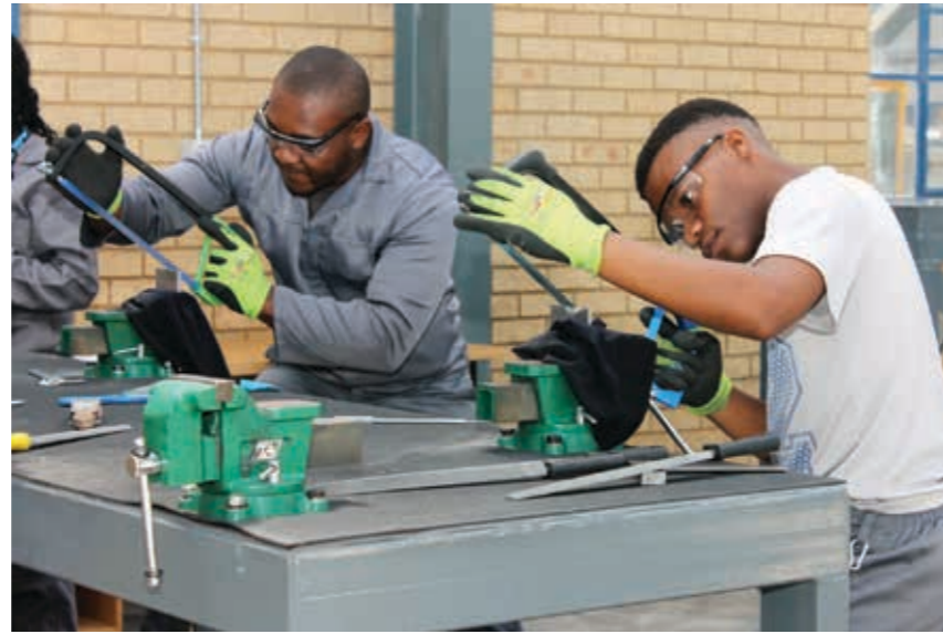
During their first year, apprentices practice the manual skills of their trade: measuring, marking, sawing, filing and drilling.
