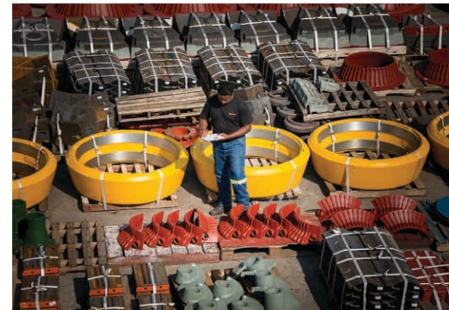
As well as its renewed focus on mill liners for fully autogenous grinding (FAG) mills, Mitak routinely manufactures and supplies high-value HCWI grinding parts such as slurry and dredge pump spares and chute linings.
