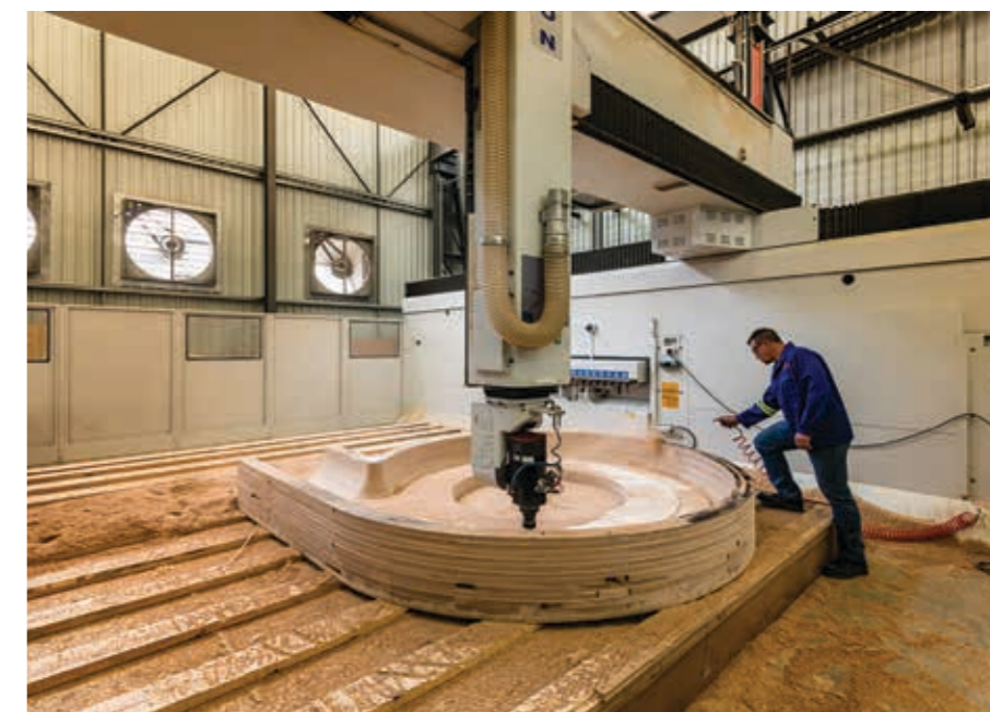
Mitak has a 5×6×2 m CNC milling machine that can automatically produce timber patterns from a product tool path for making sand moulds.
