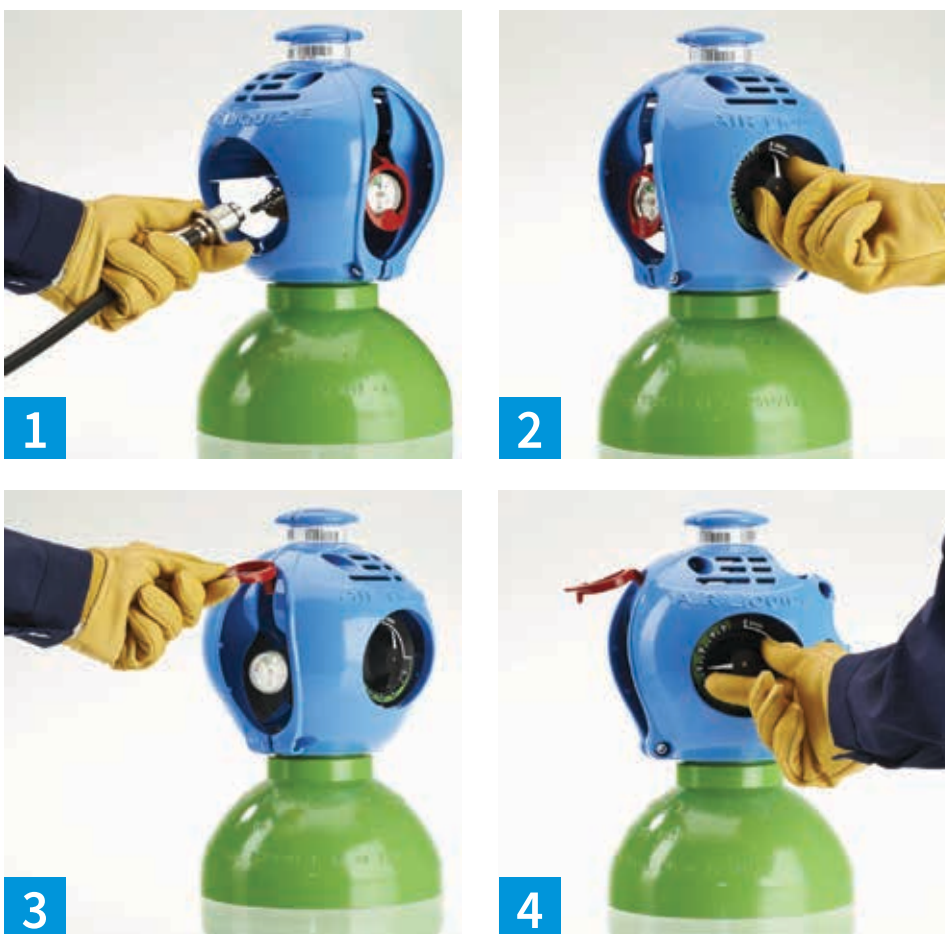
The key innovations built into Air Liquide's EXELTOP solution include: 1: A quick connector to couple the gas hose to the EXELTOP gas cylinder; 2: Easy dial setting to set the initial flow to zero. 3: A pull up lever to open the cylinder. 4: Easy flow adjustment on the graduated hand wheel.
